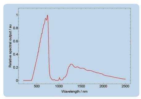
Figure 1: Relative spectral output of PSL Classic
